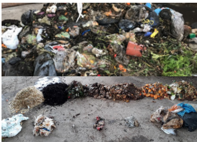
Figure 5.9 An example of a sorting analysis of collected organic waste. The picture at the top shows the waste before sorting; the picture at the bottom shows the waste after sorting (Almere).
